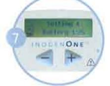
Set the flow setting to the flow rate prescribed by your clinical professional. The flow setting can be changed by pressing the triangular flow setting buttons that are marked with "+" and "-" symbols. Position the nasal cannula on your face and breathe normally through your nose.
